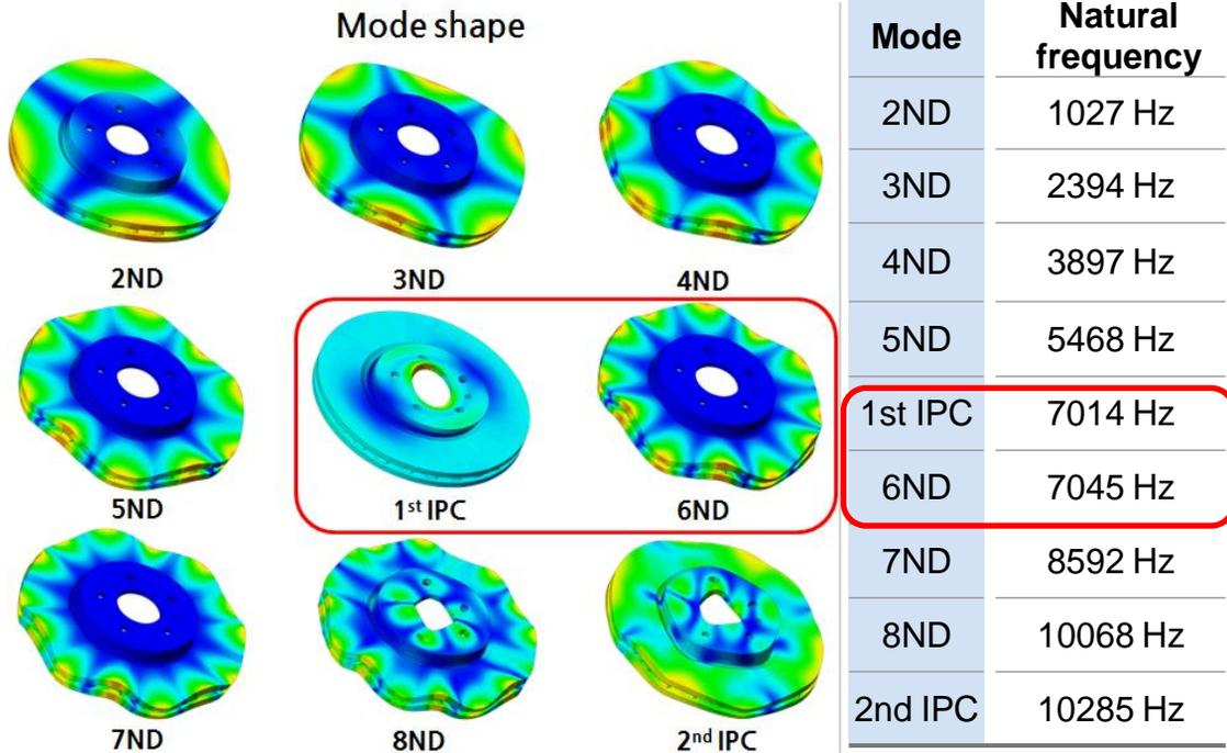
Above results are performed by midas NFX mode analysis. From the result we can see that frequency difference between 1<sup>st</sup> IPC mode and 6<sup>th</sup> ND mode is only 30Hz. The difference is too small and squeal noise is highly possible to occur. Therefore a design modification is in need for the above case.
