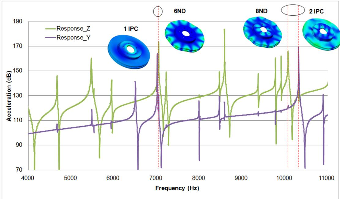
Main cause of squeal noise is indentified as ND mode (Nodal Diameter Mode) and IPC mode (In-Plane Compression Mode). ND mode is when disk shake up and down, while IPC mode is when squeezing force applied to the same side to make the disk deform.
