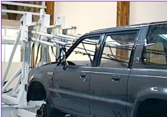
Figure 1.1 Loading device of ECE R14 test
