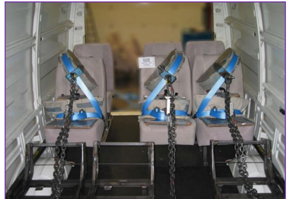
Figure 1.2 Seat belt anchored to loading device
