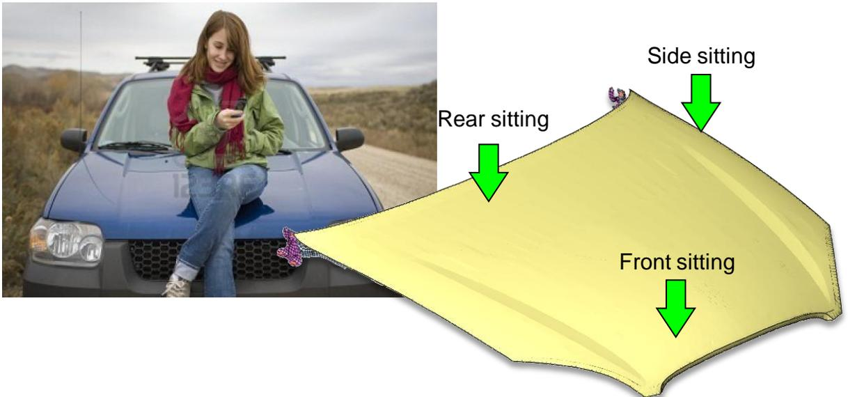
In this case we consider a situation that a person sit on the hood of his car. In order to prevent permanent deformation, car hood should reach certain stiffness. For a general case, we assigned load to front, rear and side part of the car hood respectively and check if there's permanent deformation.
