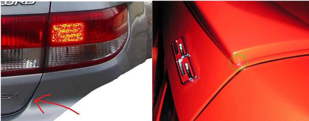
In this case, vibration occurs when vehicles drives on unpaved road . Paint on the door or body will be removed and tail lamps will interference with one another due to vibration. To prevent this situation, a simple linear analysis is used to insure minimum stiffness of the trunk.
